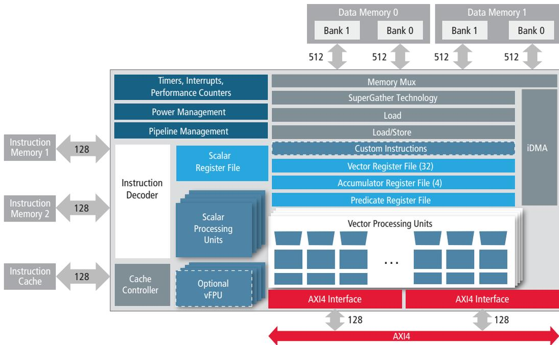
Figure 3: Tensilica Vision P5 architecture
