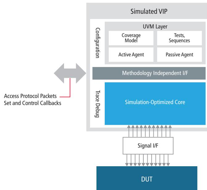
Figure 3: Simulated VIP architecture
