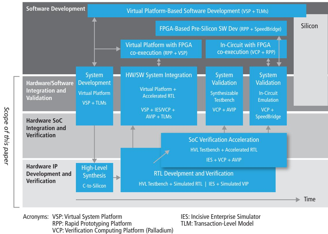
Figure 1: System development flow with mapping to Cadence verification solutions
